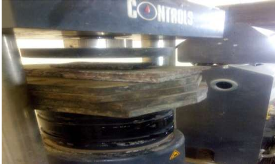
Fig 6: Sample undergoing compressive strength test
