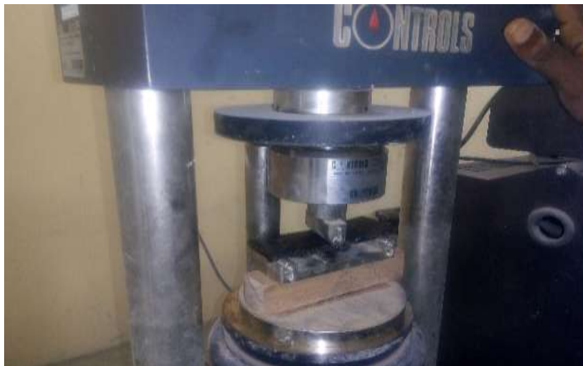
Fig 5: Sample undergoing flexural strength test
