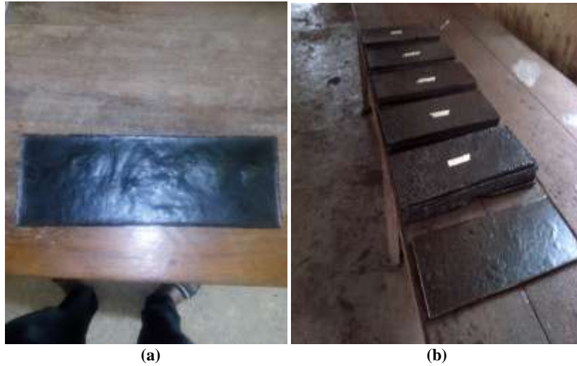
Figure 4: (a) plastic tile immediately after casting, (b) plastic tiles arrange according to sizes of reinforcement.
