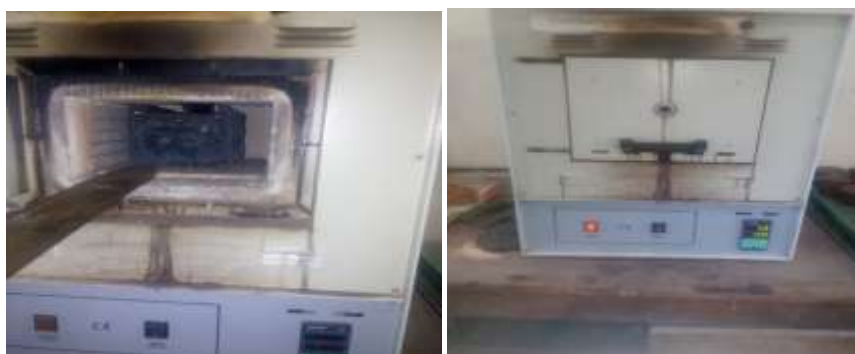
Fig 3: crucible inserted into the electric furnace and the furnace turned on at a temperature of 150
