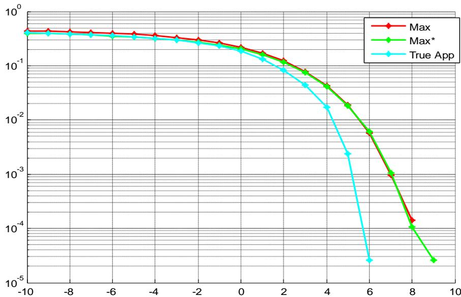
Figure 7.10 BER Comparisons between different decoding techniques for turbo code with QAM modulation over AWGN channel
