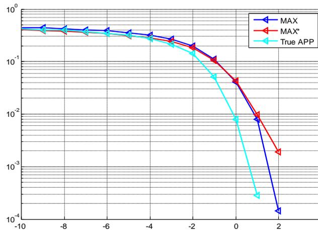
Figure 7.9 BER Comparisons between different decoding techniques for turbo code with QPSK modulation over AWGN channel
