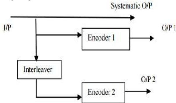
**Fig 2:** The Turbo Code encoder. [4]
