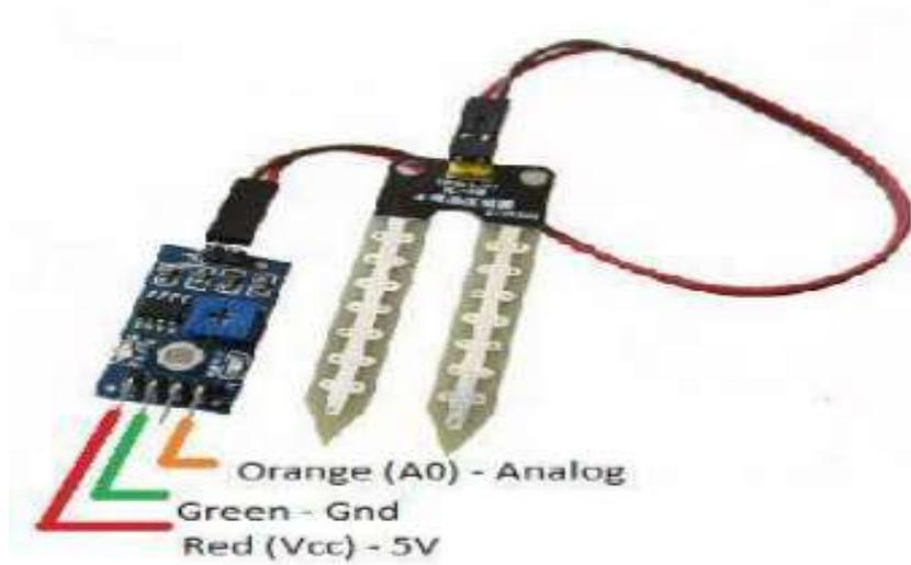
Fig. 2 Soil sensor
