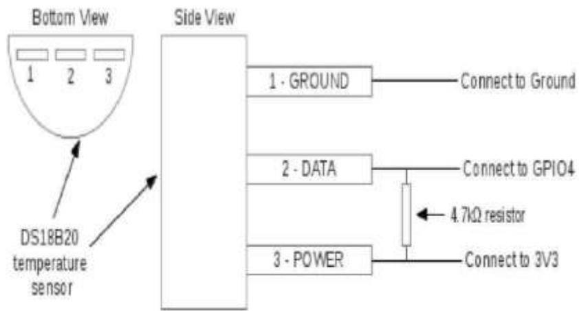
Fig.1 Block diagram of temperature sensor
