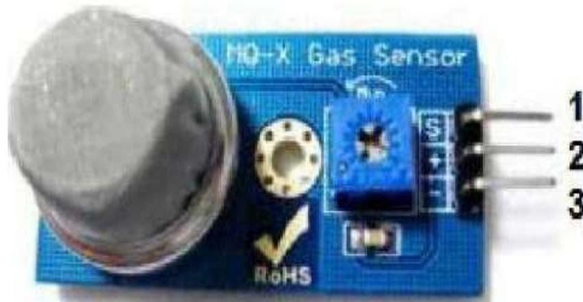
Fig. 4 MQ2 gas sensor
