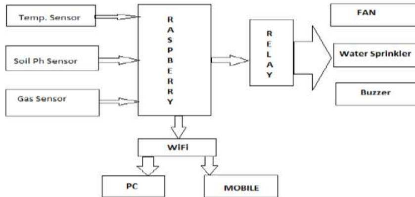
Fig. 6 Block diagram of data acquisition system for remote monitoring and controlling of soil environmental parameters.
