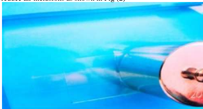
Figure 2: 200 gm weight positioned on the top of composite to remove excess material.
