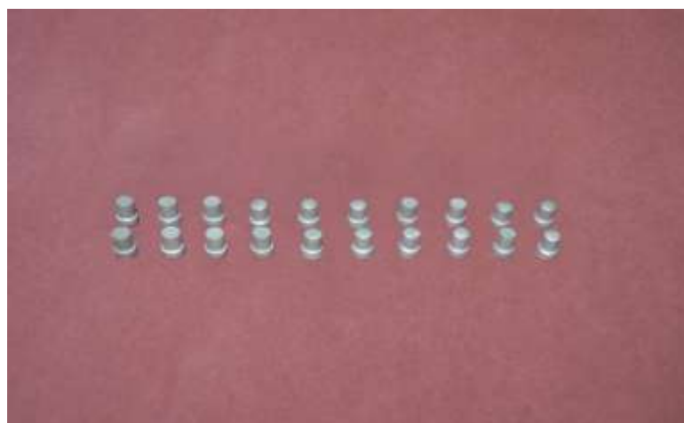
Fig.3: Samples obtained using laser sintering
