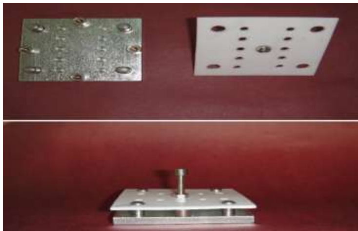
Fig.4: Metal die for ceramic build-up
