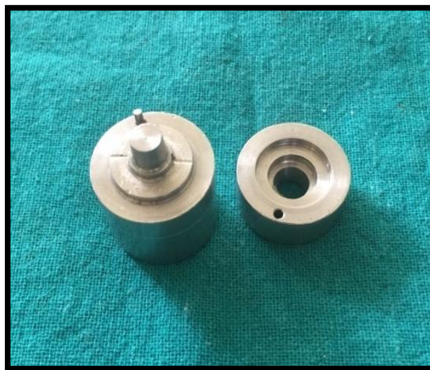
Figure 1 :Stainless Steel DieWith Metal Sleeve
