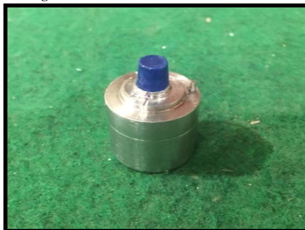
Figure 2 :Inlay Type B Pattern Fabricated On Die
