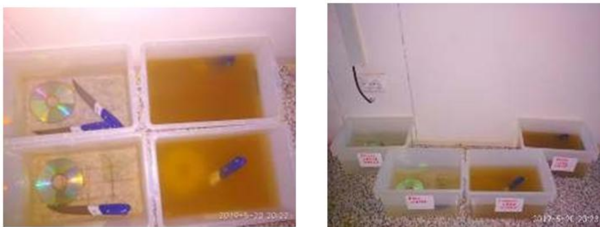
Figure 2: Non-porous surfaces were placed in Plastic tank filled with 4 type of water samples after fingerprints deposition
