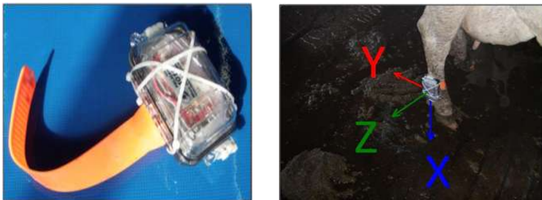
Figure 2. KinetaMap assembly (a) rugged electronic device and (b) attached to a cow
