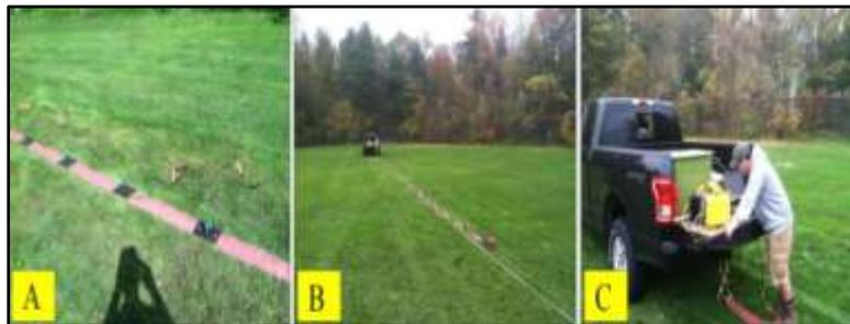
**Figure 3.** A) Close-up of base plates and geophones, B) The seismic streamer, C) The seismograph and field laptop are carried on the bed of the truck.
