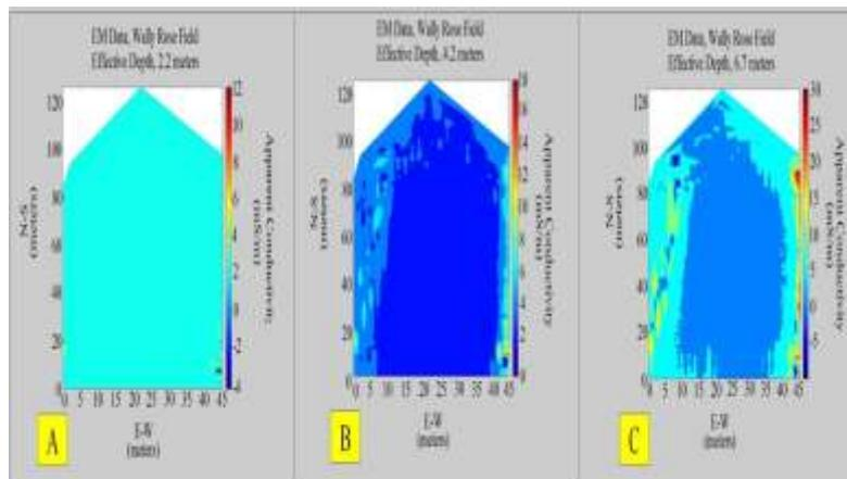
Figure 8. A) EM data effective depth of 2.2 meters, B) EM data effective depth of 4.2 meters, C) EM data effective depth of 6.7 meters.
