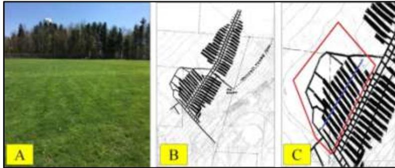
**Figure 2.** A) Wally Rose Field on the campus of Slippery Rock University, B) Historic map of abandoned coal mines beneath university property, C) Portion of abandoned coal mines beneath the study area. The location of the electromagnetic survey is outlined in red and the surface wave survey line is shown in blue.
