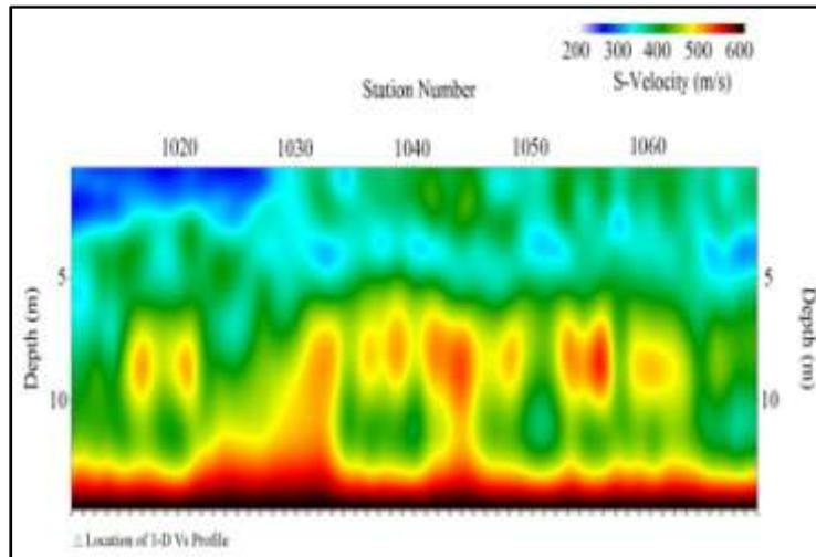
Figure 6.2-D shear wave velocity profile.
