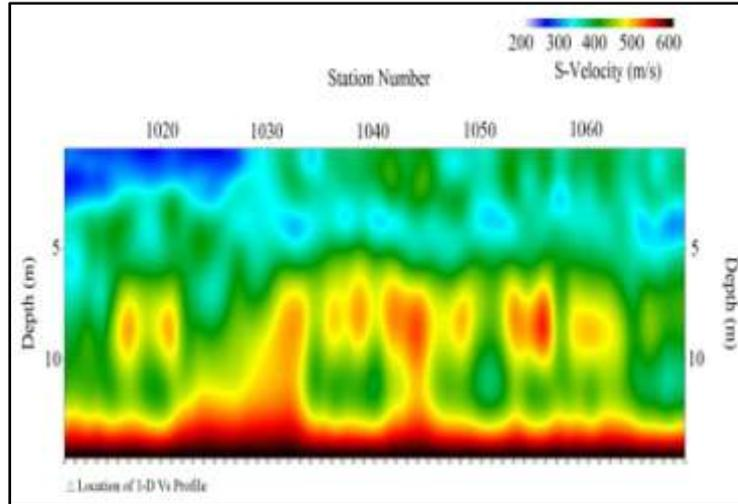
Figure 6.2-D shear wave velocity profile.
