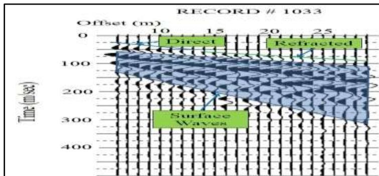
**Figure 4.** Seismic shot record from surface wave survey.
