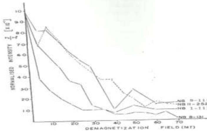
FIG. 4C: NORMALISED DEMAGNETIZATION CURVES FOR PILOT SPECIMENS OF NGONG BASALTS.
