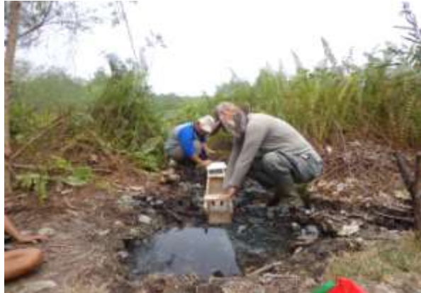
a. The styrofoam velocity measurement on the flow of the hot springs-1.
