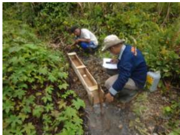
d. The styrofoam velocity measurement on the flow of the hot springs-4.
