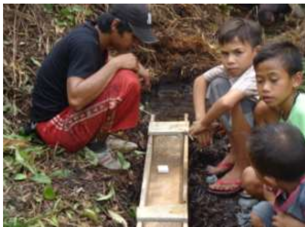
c. The styrofoam velocity measurement on the flow of the hot springs-3.
