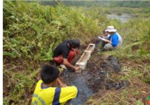
b. The styrofoam velocity measurement on the flow of the hot springs-2.
