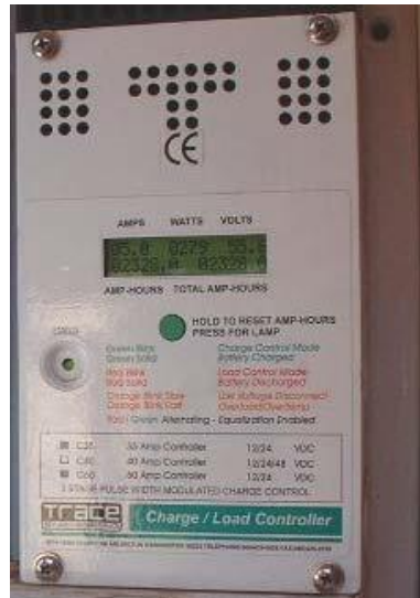
Fig 3: Front view of a typical Charge Controller
