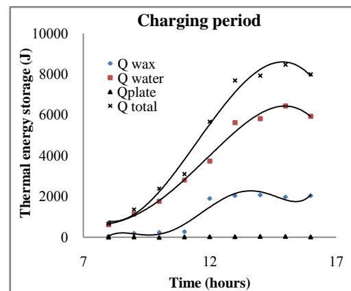
**Fig. 4,** the average thermal energy storage of the Trombe wall parts during the charging period
