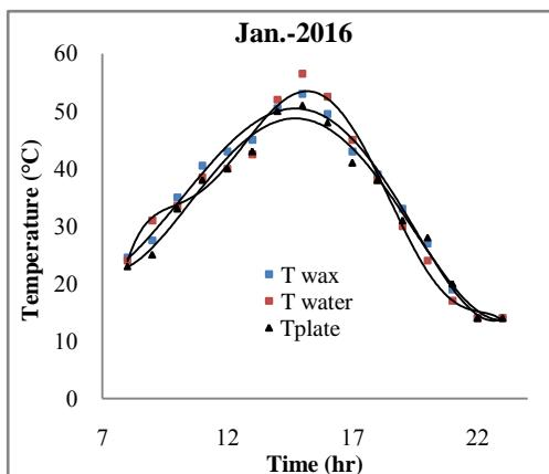
**Fig. 3,** the temperature of the Trombe wall parts during January test period
