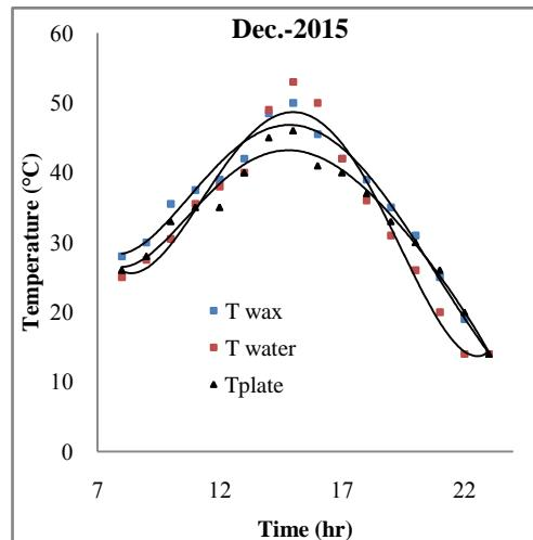
**Fig. 3,**the temperature of the Trombe wall parts during December test period
