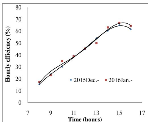
**Fig. 5,** the average hourly efficiency of the Trombe wall for the tested period
