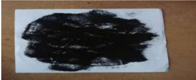
Figure 3: Iron particles (diameter 0.013mm) used for the experiment
