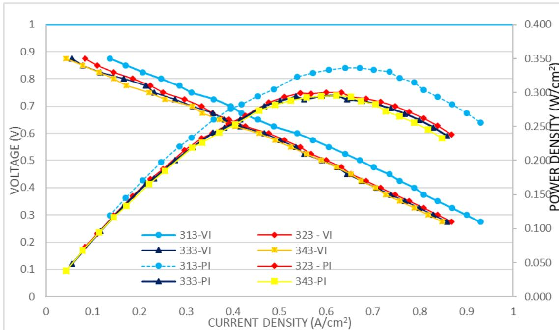
Figure 2. P-I and V-I curve of L:C – 1:2 of interdigitated flow channel with 16 cm<sup>2</sup> active area
