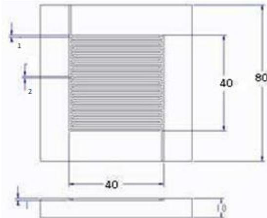
**Figure 1.** Interdigitated flow channel with Landing to channel width ratio -1:2 of PEM fuel cell
