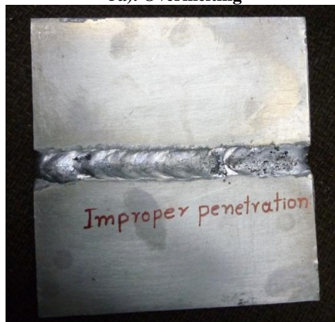
5b). Improper penetration
