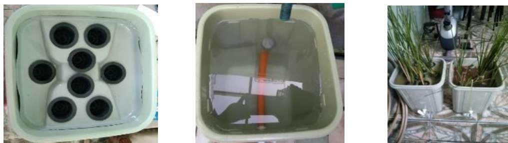
Figure 1: Phytoremediation box, Figure 2: Wetland box with media, Figure 3: Phytoremediation and wetlands complete with plants.
