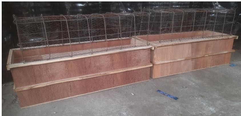
Figure 4. Reinforcement of the frame and making of the laboratory scale ferrocement mold
