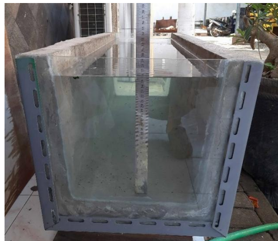
Figure 5. Observation of laboratory scale ferrocement water loss test
