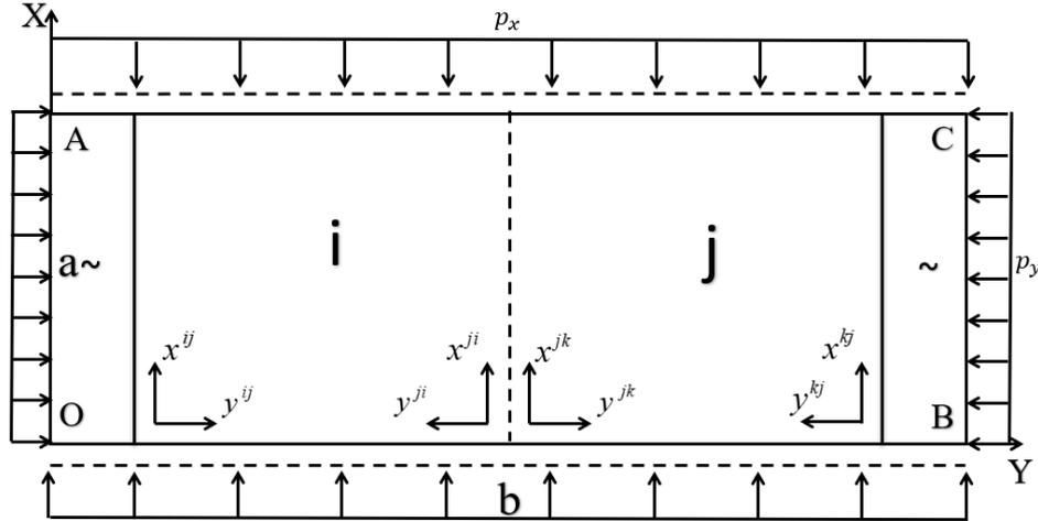
Fig. 1 Geometry and coordinate system of a thin multi-span plate
