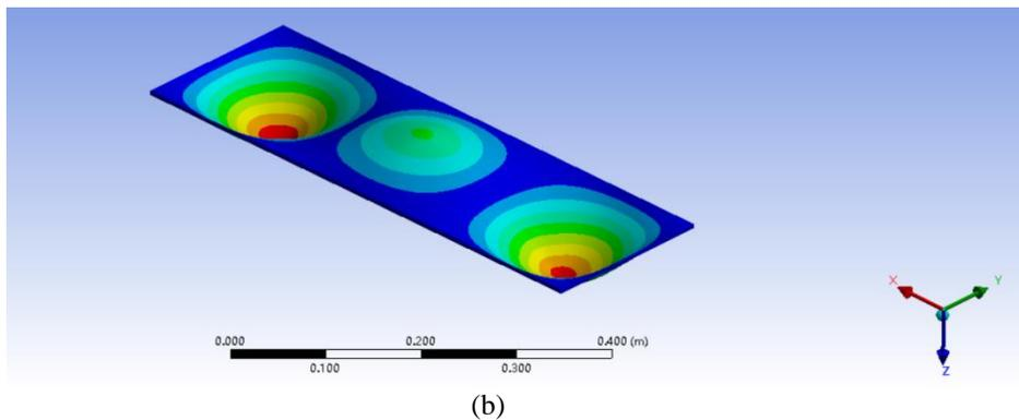
**Fig. 4** Comparison of mode of buckling (a) MRRM; and (b) FEM
