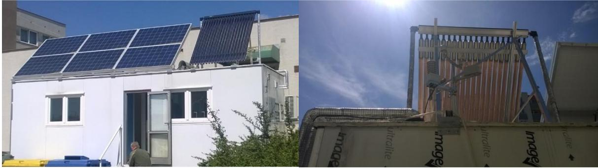
**Figure 3:** Mobile laboratory - photovoltaic and solar thermal panels, meteorological station
