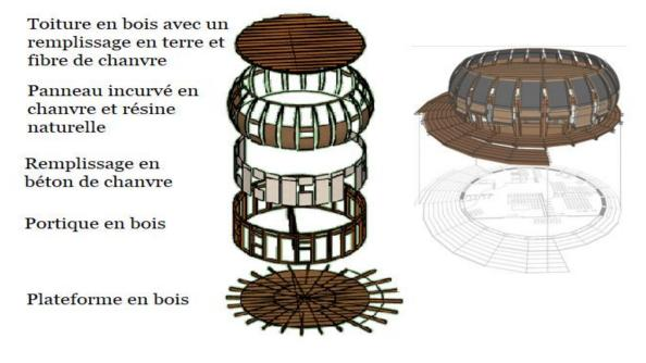
In this section, a case study is presented, it relates to the conceptualization / construction of a zeroenergy building as part of the international competition Solar Decathlon, Africa 2019. The building is designed with a circular shape that is inspired by the architectural model of traditional houses found in various African countries.
