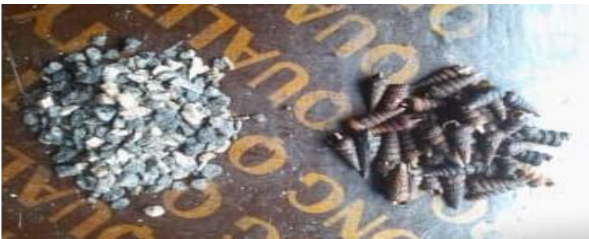
Figure 3: 9.5 mm size granite and periwinkle shells samples
