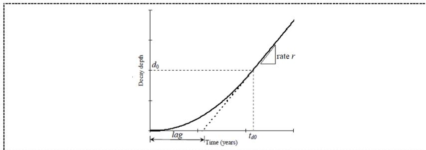
**Figure3:** Decay depth model,  $d(t)$  vs.  $t$
