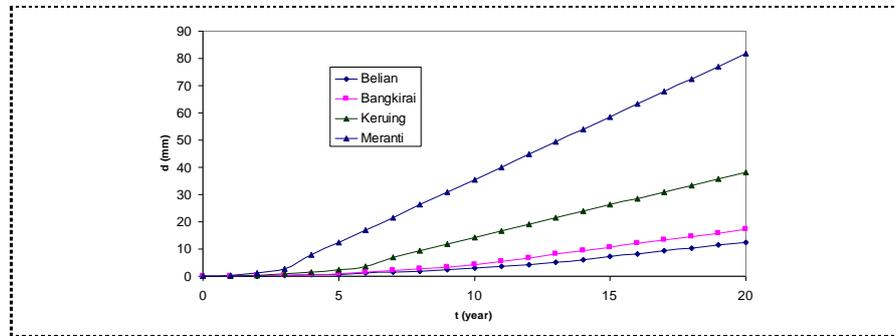
Figure5: Decay depth  $d(t)$  vs. time ( $t$ ) for above-ground decay model for different durability classes of tropical wood species
