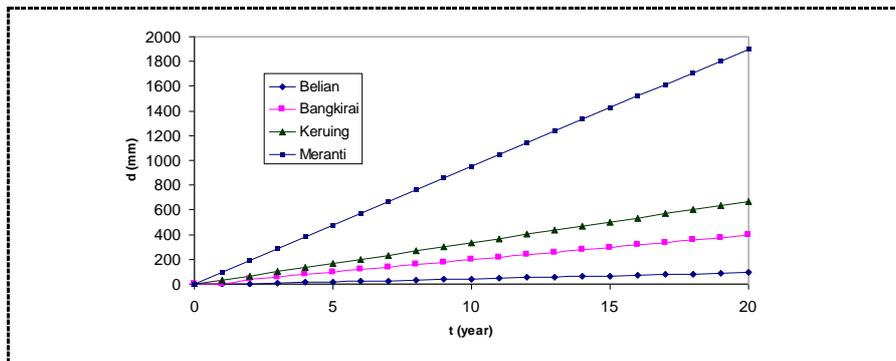
Figure6: Decay depth  $d(t)$  vs. time ( $t$ ) for marine borer attack model for different durability classes of tropical wood species
