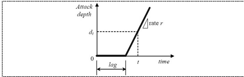
Figure 4: Decay depth model,  $d(t)$  vs.  $t$
