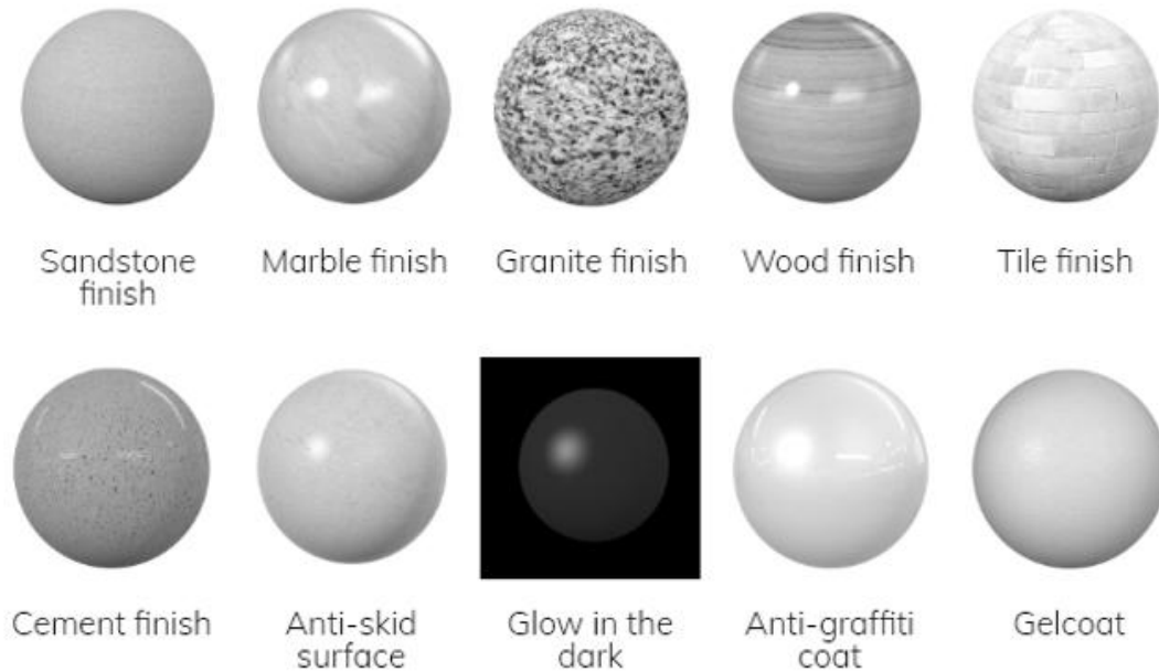
Fig. 2. The different types of natural final finishing and coloring of the FRP composite materials for architecture use [10] ( http://www.bfgarchitecture.com/building_envelopes )
