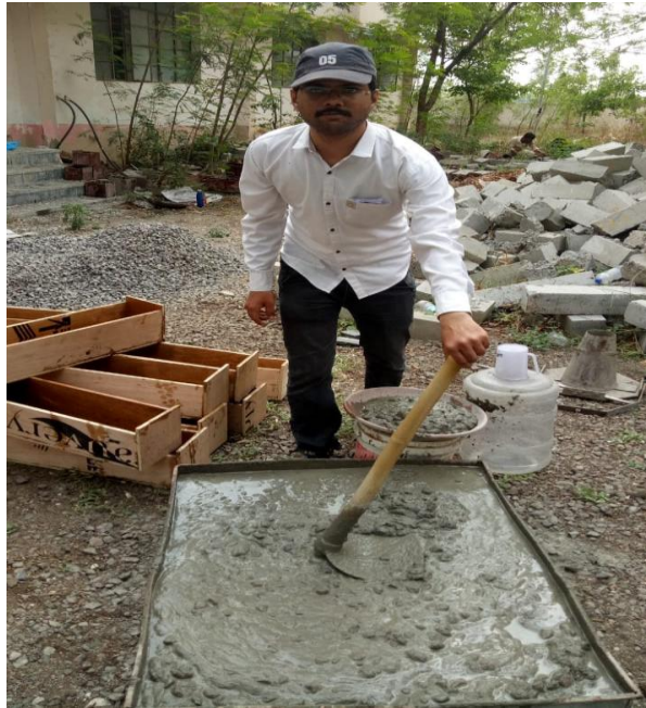
Fig. -1 Over burnt brick bats added to concrete
