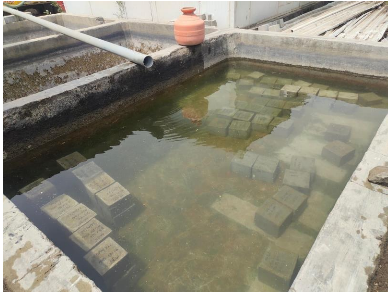
Fig 1: Curing of Cube and Beams
