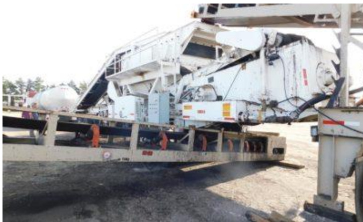
Figure Cold Central Plant Recycling (CCPR)
