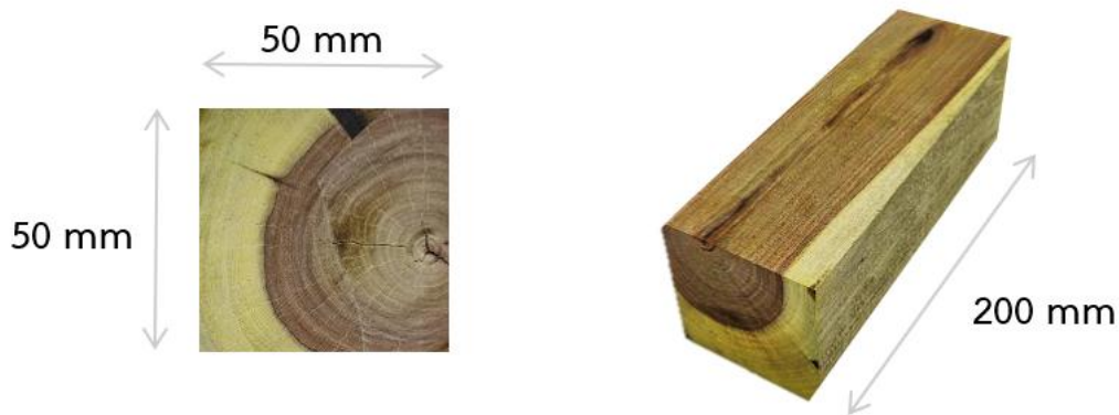
Figure 4: Burma Padauk timber specimen 50x50x200 mm: (a) top view and (b) perspective view.
