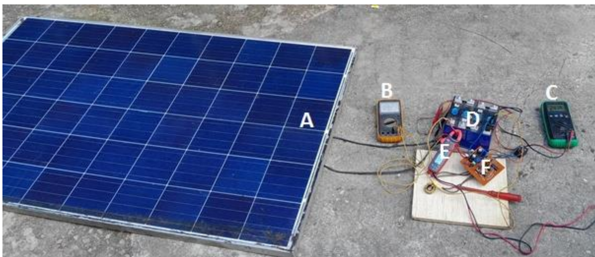
Figure 17 The Systemtest setup, (A) 260W Solar panel (B) Battery voltmeter (C) PV Voltmeter (D) Test Battery (E) PV Current meter (F) MPPT Board under test.
