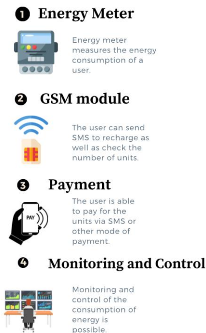
Figure 1 layout of the prepaid energy meter system
