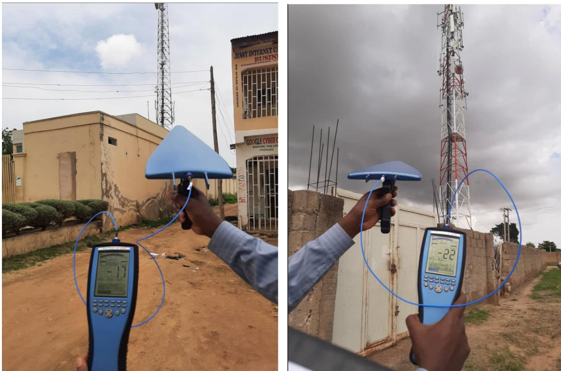
Figure 1: Measurements of the power received with Aaronia AG SpectranAnalyzer (HF-6065 V4)
