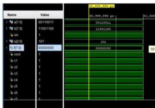
Fig 5.8 By setting S2=1, S1=0, S0=1 and Cin=1 AND operation is carried out by 64 bit proposed design ALU
