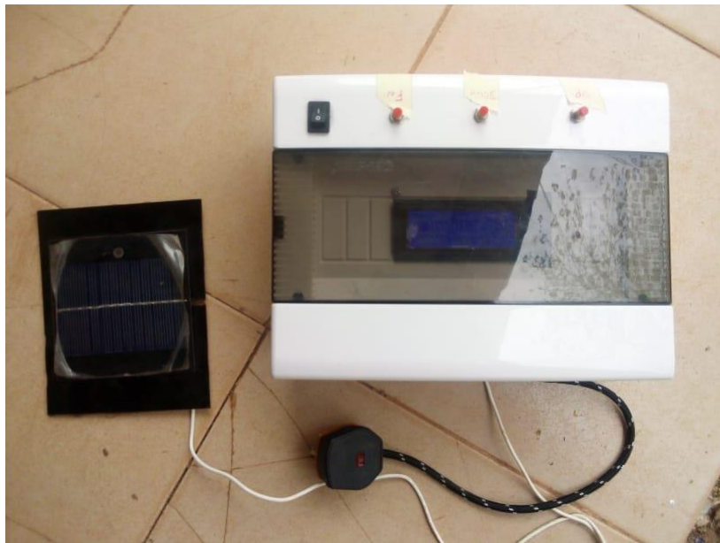
Fig. 8 External view of the developed solar data logger
