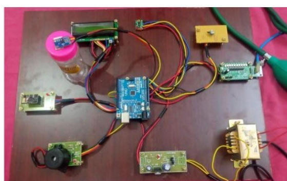
Fig.3 Patient monitoring kit using IoT
