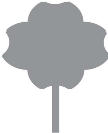
Figure 5: Flower shape antenna geometry
