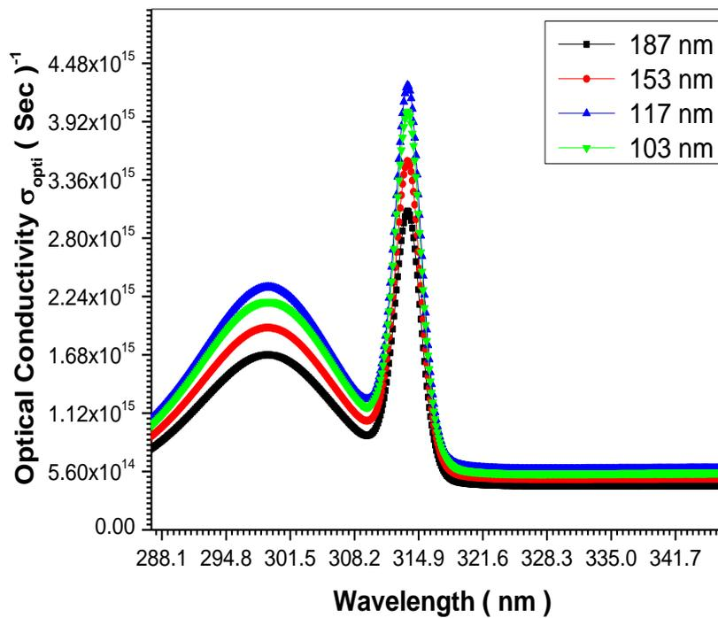
Fig (7) Plot of optical conductivity( $\sigma_{opti}$ ) as a function of photon energy for Fe<sub>2</sub>O<sub>3</sub> thin film.
