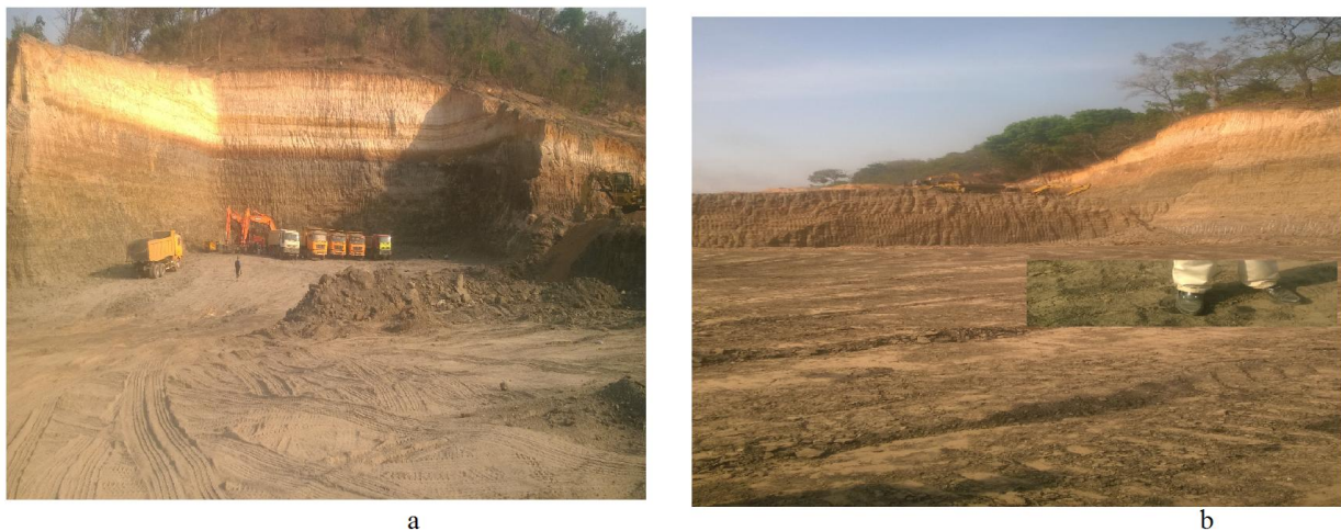
Figure 16. a, Coal Exploitation Site, Showing Machineries and Excavation (Overburden Removal) Done to Coal Point. b, New Expansion Site for Coal Exploitation, Showing Machineries and Excavation to Top-of-Coal after Removal of Earth's Overburden Material.
