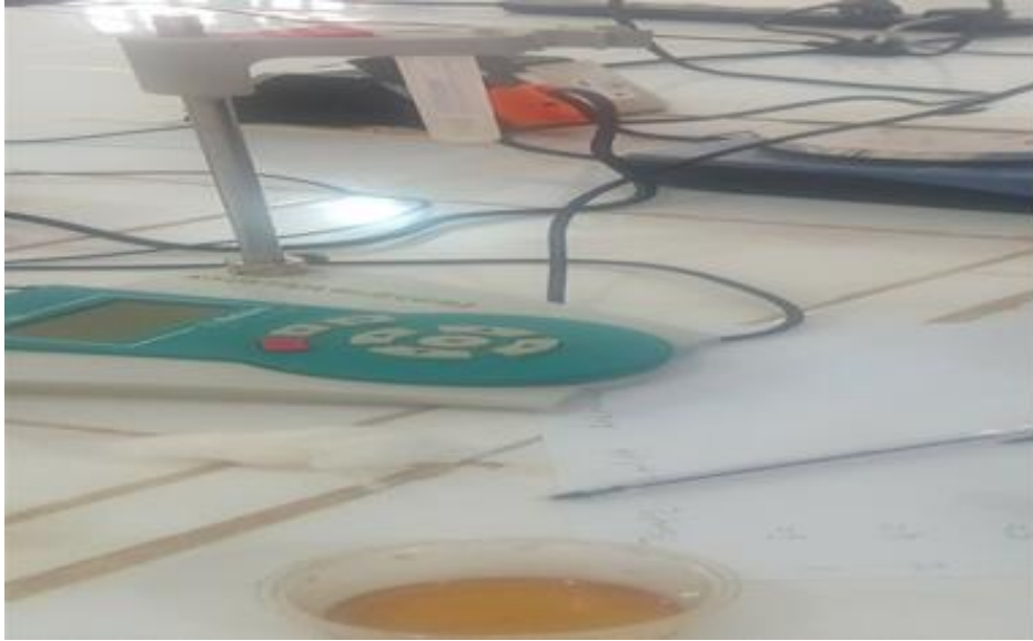
Figure 3: Set-up for Measurement of pH Values of Samples
