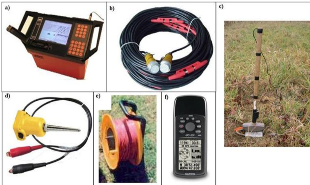
Fig. 3: Seismic refraction survey equipment. (a) Digital seismograph ABEM Terraloc MK6, (b) Seismic land cables, (c) sledgehammer (d) vertical geophone, (e) reel wire, and (f) GPS Device, (Rami, 2014)
