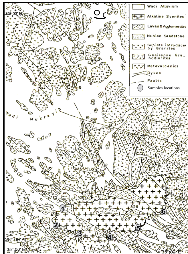
Fig. 3: Photogeological map of Gabal Nigrub El Tahtany (after El Ramly et al., 1979) and locations of the collected samples.
