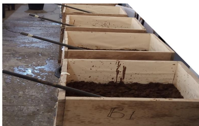
Plate 1: wooden microcosm stacked with different treatment options as presented in Table 1
