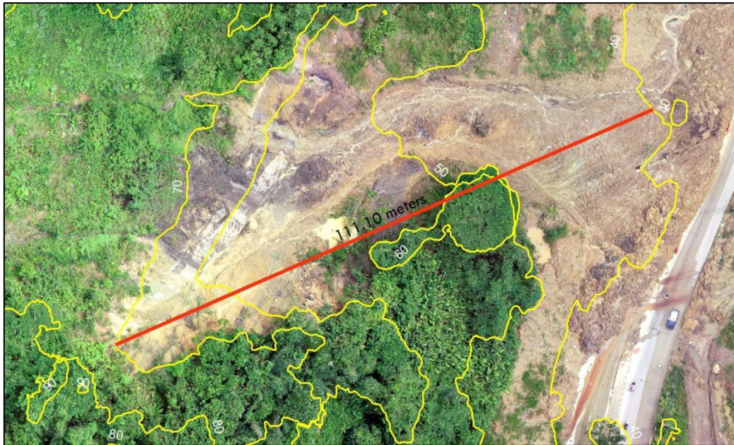
Figure 4. Flat Distance from Landslide Head to Landslide Foot
