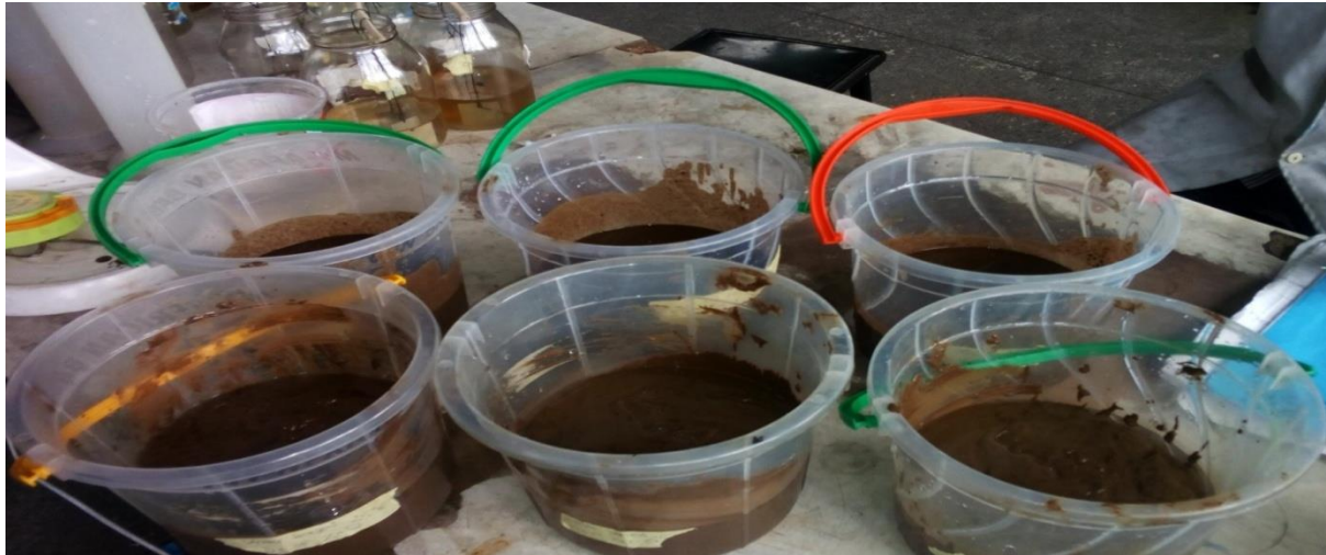
Figure 1: Water-based mud sample with different grams of coconut shell nanopowder
