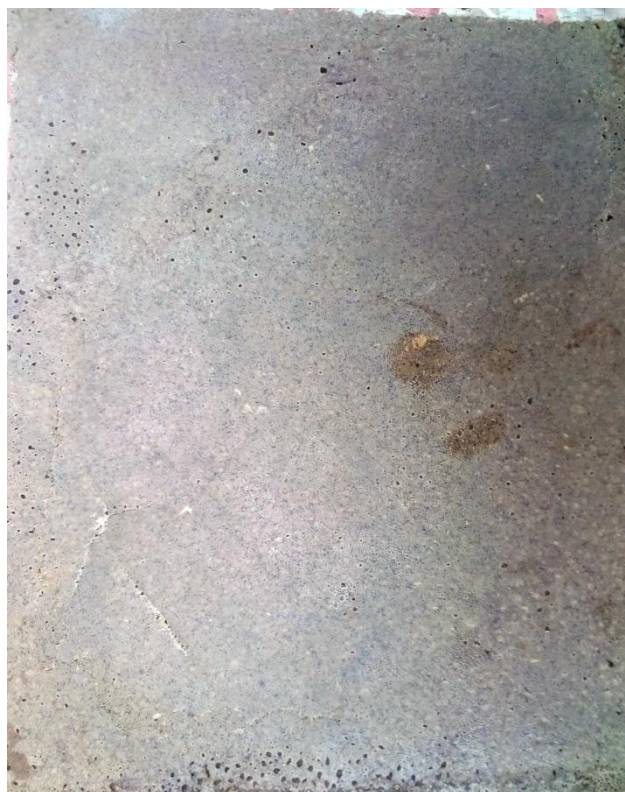
Plate 2: Plastic tile made from light colour plastic waste
