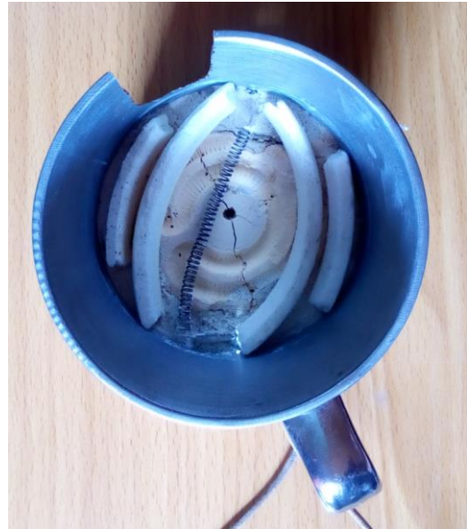
Figure 6: Mounting of the Element on the Cup
