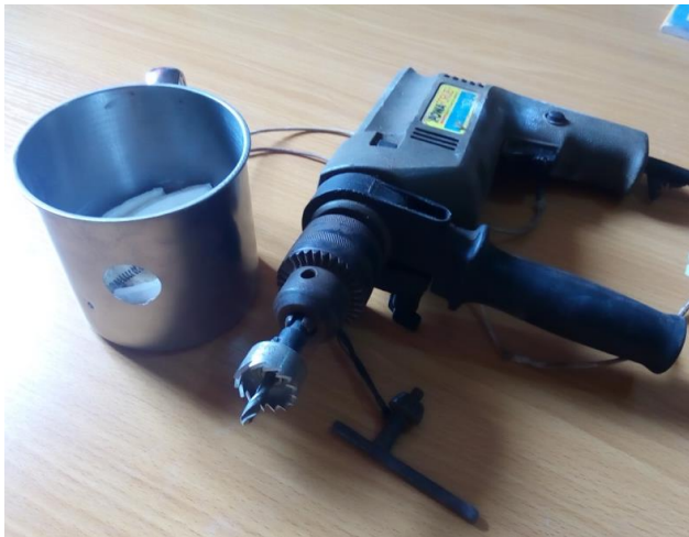
Figure 7: Drilling of Circular Hole on the Cup
