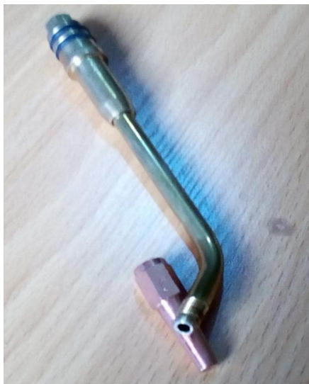
Figure 3: Gas Burner Nozzle
