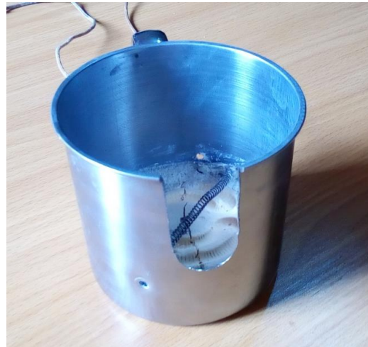
Figure 8: Cutting of the Tape space on the Cup
