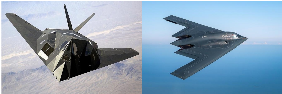
“Stealth aircraft like the F-117 Nighthawk and B-2 Spirit introduced radar-evading technology.”
