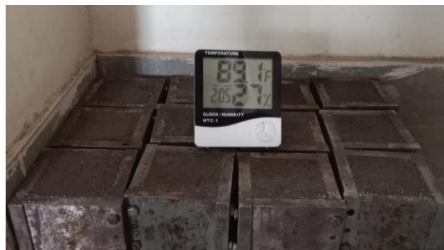
Fig. 2: Moulds Filled with Cement-Sand Mortar
