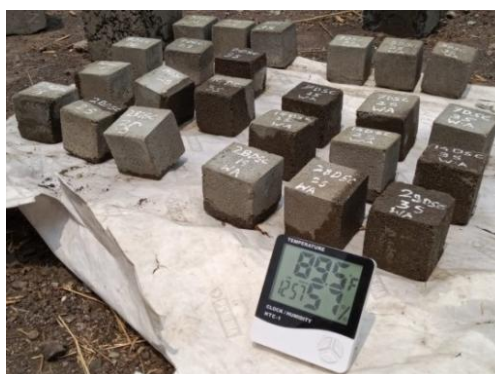
Fig. 4: Specimens Placed in the Field (Under the Sun)
