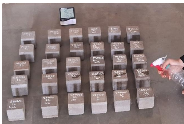
Fig. 3: Spray Curing Being Done
