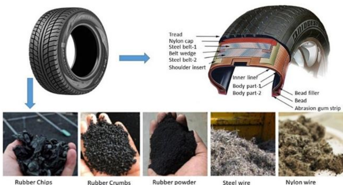
Figure 6. Schematically shows the grinding and granulation of old tires [17].
