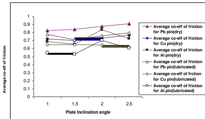
**Fig. 8(b): The dependence of Average co-efficient of friction with plate inclination angle when Pb, Cu and Al pins slid on shot blast steel surfaces**
