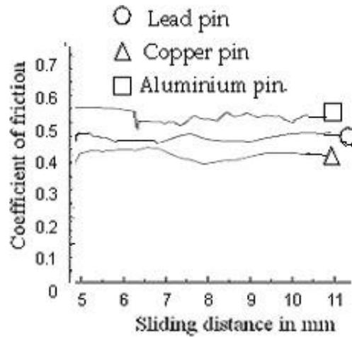
Fig. 5: Dependency of co-efficient of friction with sliding distance for ground (SiC polished) steel surface.
