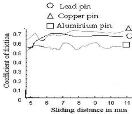
Fig.7: Dependency of co-efficient of friction with sliding distance for EDM surface
