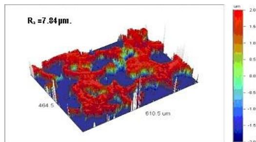
Fig.3(c): The three-dimensional view of EDM plate surface.
