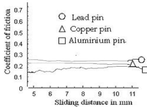
Fig. 6: Dependency of co-efficient of friction with sliding distance for shot blast steel surface.
