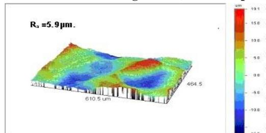
Fig.3 (b): The three dimensional view of shot blast plates surface
