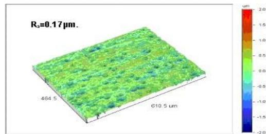
Fig.3 (a): The three dimensional view of ground (SiC wheel polished) plate surface.
