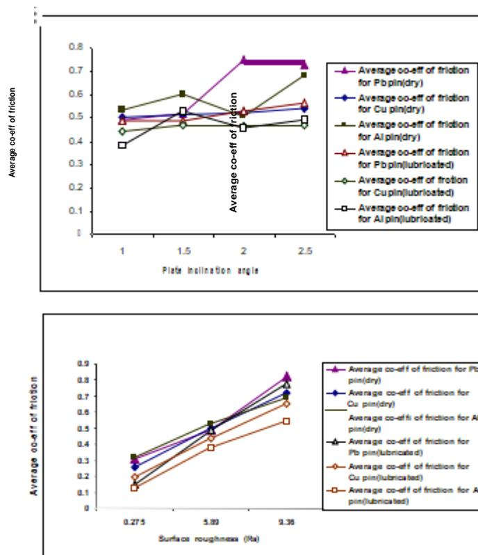
**Fig. 8(c): The dependence of Average co-efficient of friction with plate inclination angle when Pb, Cu and Al pins slid on electric discharge machined steel surfaces.**
