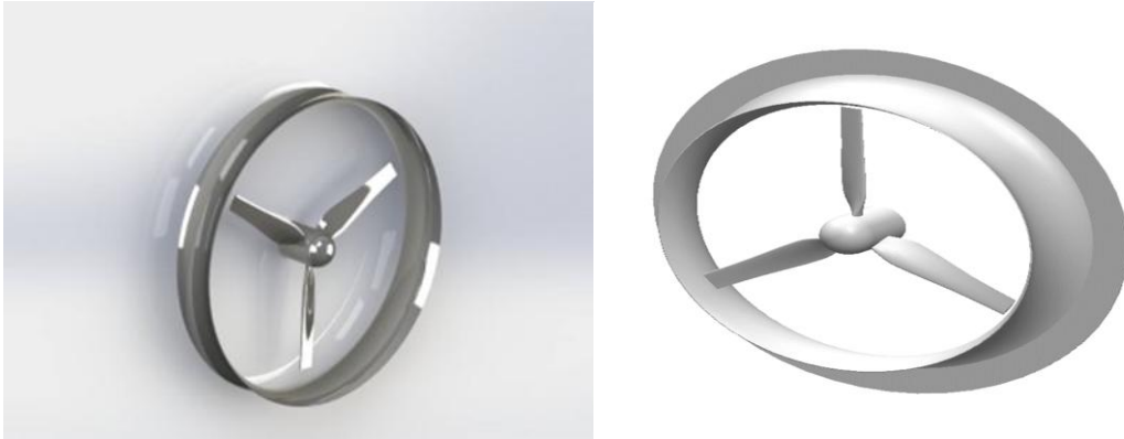
Figure 6: Wind Turbine equipped with a flanged-diffuser shroud.
